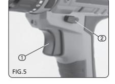
(ii) When the drill is not in use move the direction switch to the neutral position (the middle setting) to lock the trigger out. This will help prevent accidental drill operation and drill burn-out situations.
