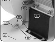
Locate the gasket (17)and the extraction chute (3) to the top of the motor and secure with 8 x M8 x 16mm bolts (11). NOTE: Ensure there is one washer (10) per bolt.
