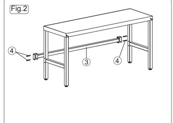
**4.3.** Stand the workbench onto it's legs. Locate and fit brace to the rear legs using four hex bolts. The workbench is ready to use.
