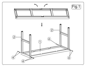
**4.2.** Lay the table top face downwards. Insert one H frame into the grooves at one end of the table top and fix in place using 4 hex bolts. Repeat wit the other H frame.
