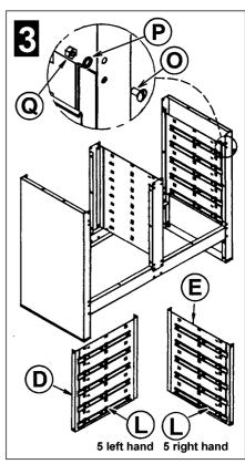
STEP 3. Bolt left & right slide panels (D) & (E) into position using 8 bolts (O), 8 lock washers (P), and 8 nuts (Q). Fix 5 left hand female slides (L), onto slide panel (D) and 5 right hand female slides (L), onto slide panel (E) Refer to Diagram 11 on how to fit slides.
