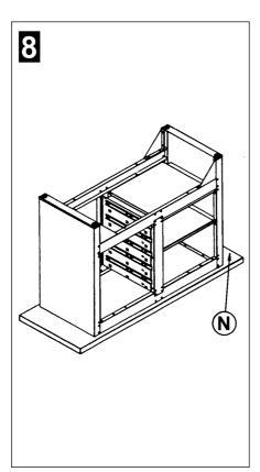
STEP 8. Place the wooden top (N) face down on a flat, clean, smooth surface. Place the cabinet upside down on the wooden top and align it with the four pre-drilled holes. Fix with the four hex head screws (S).
