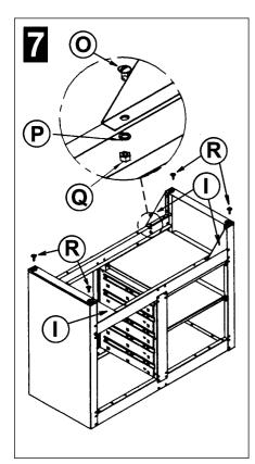
STEP 7. Turn the cabinet upside down and screw in the four adjustable leg levellers (R). Bolt the four corner braces (I) into position using 16 bolts (O), 16 lock washers (P), and 16 nuts (Q)
