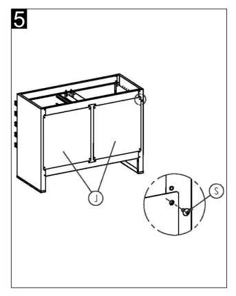
**STEP 5**. Secure the back panels (J) using 8 screws, 4 in each corner.
