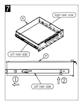
**STEP 7**. Attach the inner slides onto the drawers. Slot the horizontal tab into the hole in the drawer and the vertical tab into the other hole. Push down until the stop slots into the small hole.
