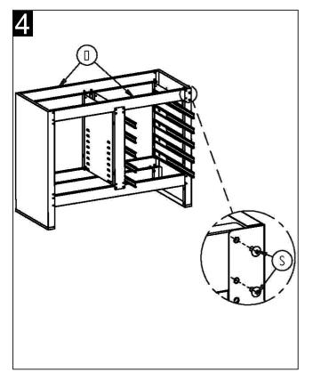
$\ensuremath{\text{STEP 4}}$  . Screw the top rails (D) onto the front and back.
