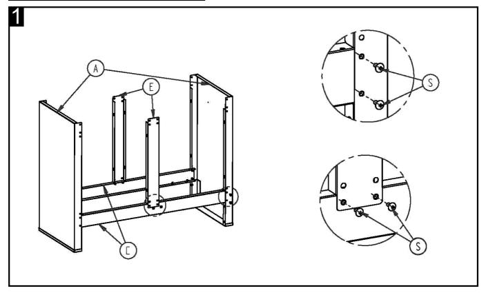
Step 1. As shown in the diagram assemble the two large side panels (A), bottom rail (C) and centre support (E).
