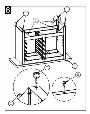
STEP 6. Turn the workbench upside down and screw in the corner braces (O) as shown in the diagram. At each corner attach the leg levellers (T). Slide the workbench top (P) under the main unit and fix with 4 hex head screws (U)
