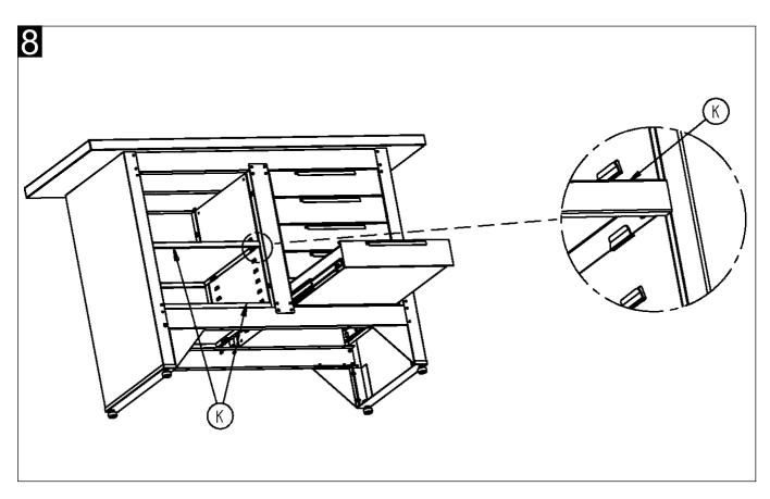
STEP 8. Pull the middle slide and the ball bearings out as far as possible. Hold the drawer and slot the inner slide on the drawer into the middle slide, then push the drawer all the way in. take the shelves (K) and slot them into the support panels at the height required. To remove drawer see Step 2.
