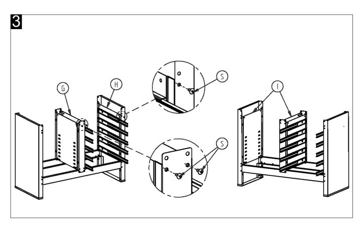
Step 3. Attach the side panels (G ,H) onto the main unit by screwing them to the front centre support (E) and side panels. Attach support panels (I) to the side of the unit without sliders.
