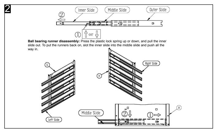
STEP 2. Attach the outer slide to the corresponding left/right side panel (G, H). Insert the tabs into the holes in the side panel making sure that the slider stop fits into the small hole.
