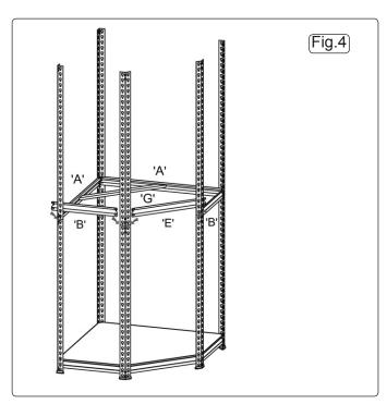
4.5. Fix shelf brackets A so that the top rivet sits in the upper legs and the lower rivet sits in the lower legs. Repeat with shelf brackets B and E, followed by brace G, at the same level.
