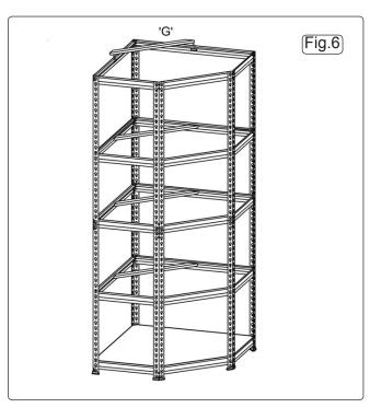
4.7. Apply remaining brackets at desired heights, ensure a brace G is also fixed at each shelf height.
