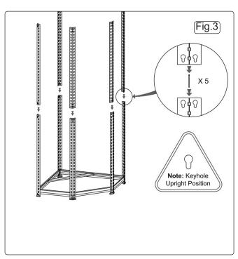
**4.4.** Join the lower and upper legs with the connector pins as shown in Fig.3 (note the upright position of the keyhole).
