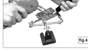
3.19 'Prime' the sucker by pushing the plunger down until it latches. Bring the soldering iron or gun to the joint and melt the solder. As soon as
