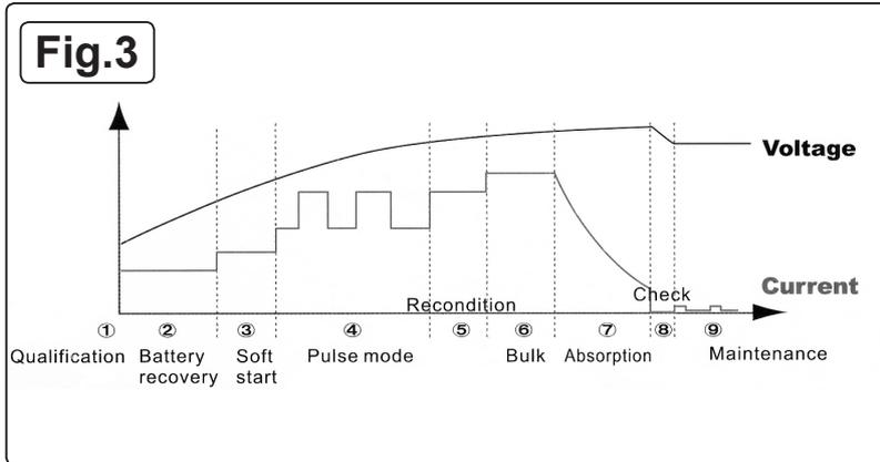
6.1. The **SMC02.V2** charger has a nine step fully automatic charging cycle as shown in Fig.3 above, which is indicative of the typical charging curve for a battery.
