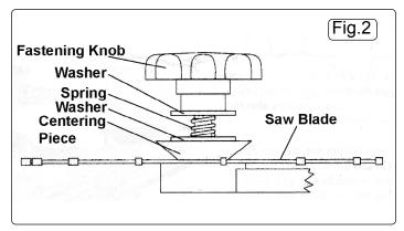
4.3. The saw blade only needs to be centred but not tightly fixed. Screw down the fastening knob only as much as necessary for sufficient tension, so that the saw blade can still be turned. Make sure that the centring piece is not slanted. (See fig.2). Original Language Version (© Jack Sealey Limited )
