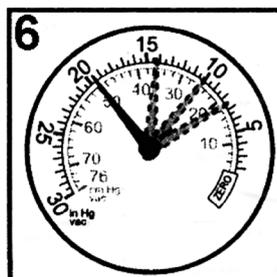
READING: Regular fluctuation between normal and low readings.
