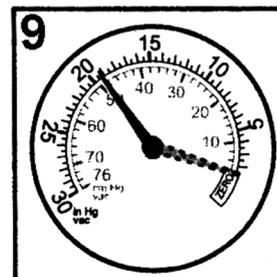
READING: Normal when first started but drops rapidly when revs held at 3000rpm.
