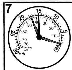
READING: Readings slightly lower than for normal engine including when throttle is suddenly opened then released.
