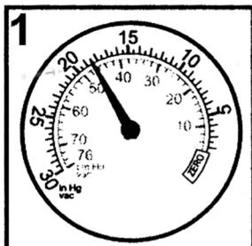
READING: 16-21 inHg with needle steady.
