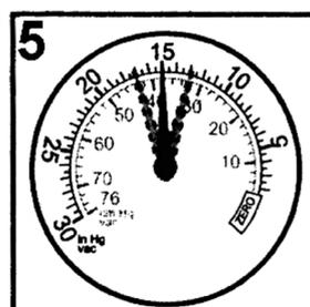
READING: Reading slightly low and fluctuating slowly.
