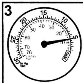
READING: Reading extremely low but steady.
