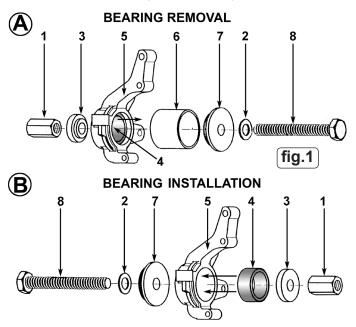
**BEARING INSTALLATION:** Identify the correct sleeve cap (7) to sit on the outside of the bearing housing and the correct diameter drift (3) to drive the new bearing into the housing. Assemble as shown in fig.1B. Keep the hub screw and nut well lubricated whilst driving the new bearing into the housing.
