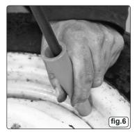
3.2.5 Use the push/pull driver to force the tyre valve all the way through the cone until it has entered the wheel (fig.6).
