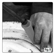
3.2.4 Place the thin end of the cone into the valve hole in the wheel rim and align the tyre valve (fig.5).
